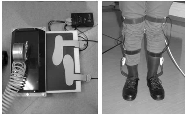
Fig. 16. The insoles are 2.5 mm thick and consist of an array of 99 capacitive pressure sensors distributed across the insole
