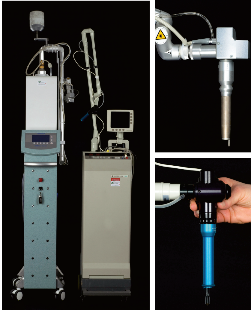
Figure 4. Carbon dioxide lasers with microprocessor controlled scanners.
