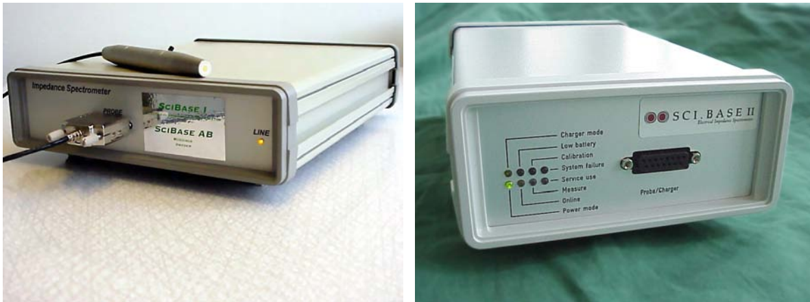
Figure 25. The SciBase I (left) and II (right) depth resolved impedance spectrometers used in the studies.
