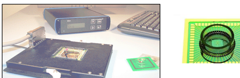
Figure 5. Microelectrode array heating system and culture dish.
