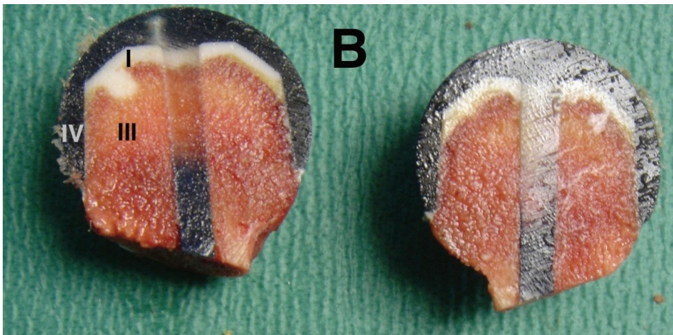
Figure 6. Photographs of the surface of a saw cut showing the regions of interest. Group A with low viscosity (LV) cementing and group B with high viscosity (HV) cementing.
