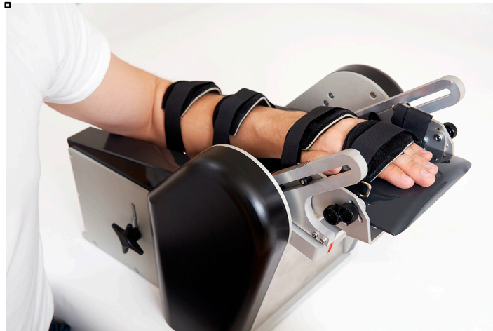
Figure 4. The NeuroFlexor measurement device used in Studies II–IV. A PC is connected to the device to control the measurements, store the data, and perform the analyses. Photo: Ola Gäverth.
