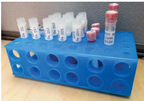
Figure 9. “In-house-produced” test-tube phantoms containing known masses of calcium hydroxyapatite (CaHA).
