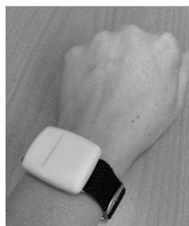
Figure 8. The GENE-monitor is a small tri-axial accelerometer measuring vertical, anteroposterior and mediolateral movement.
